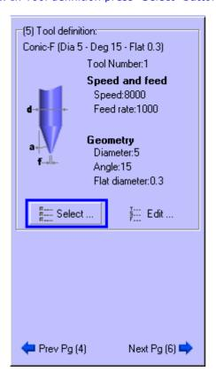
12. Click in the Tool List to select the tool. Set feed and speed of the tool. Press the "OK" button.
