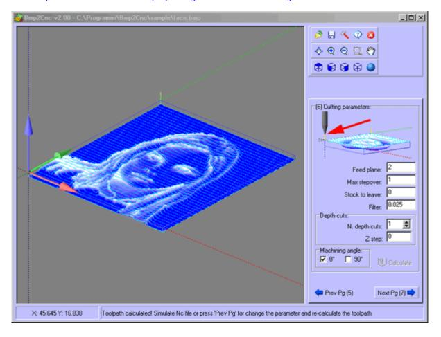
17. Turn Off the shading: only the toolpath will be displayed.
