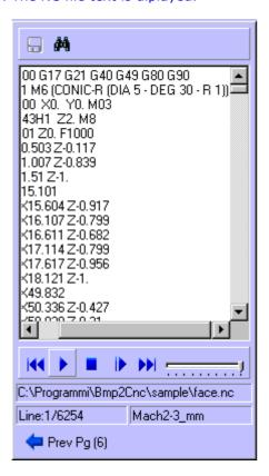
20. Press the "Play" button to simulate the toolpath (Yellow=Rapid, Cyan=Feed).
